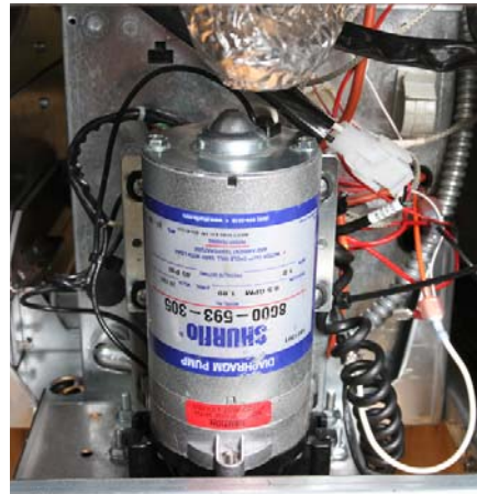
Figure 12: Route the heater controller wire over the pump and to the right.
