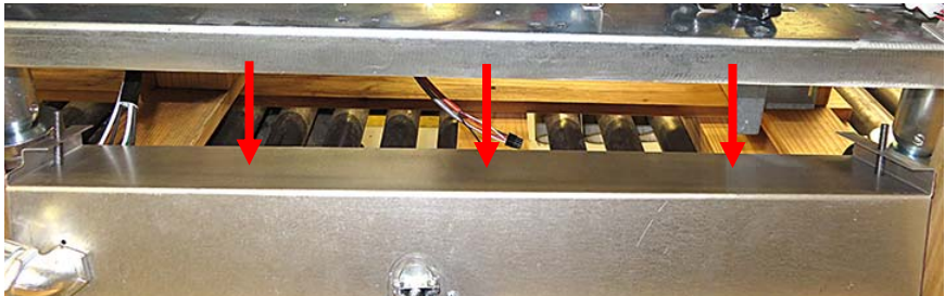
Figure 19: Transformer box lowered from the fryer.
