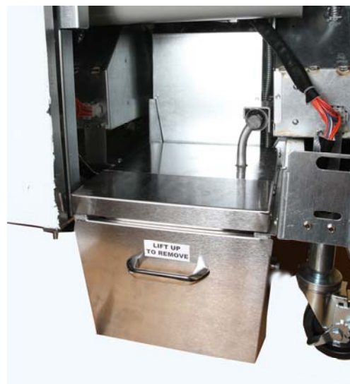
Figure 29: The heated JIB platform is shown in place with the metal JIB.
