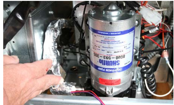
Figure 16: Route the wrapped flex line to the pump inlet side.
