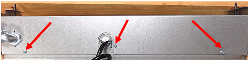
Figure 20: Remove the three sheet metal screws to remove the cover.
