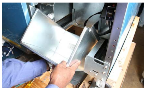
Figure 10: The heated JIB platform must enter the JIB cabinet at a steep angle.
