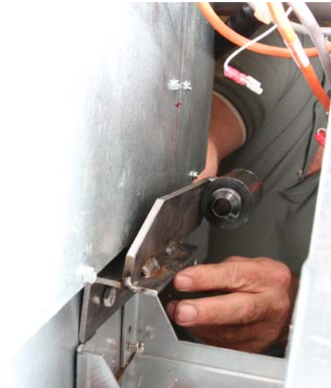
Figure 4: Positioning female oil pickup on fryer channel using the 1/4 x 20 bolts securing the pickup. May not be necessary in newer fryers.
