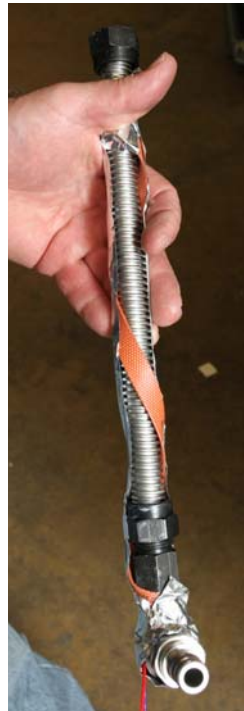
Figure 17: Position straight or gradually wrap the provided, larger diameter, inlet and outlet flex lines with heater tape. Ensure the wire leads exit near the junction box position.
